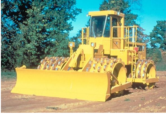
Figure 20: CAT sheepfoot roller
